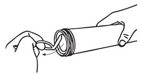
Only then tear off the cartridge's "pull-off" closure and screw on the grease gun head.
