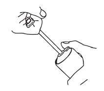
Pull on the push rod, actuate the safety catch, and push the push rod back into the cylinder.
