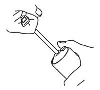
While pulling on the push rod, activate the safety catch and push the push rod back into the cylinder.
