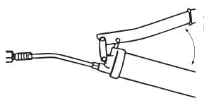
Actuate the hand lever to carry out the greasing process.
