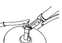
Place the grease gun onto the filling valve of the grease gun filling unit, and hold it in place with light counter pressure.
