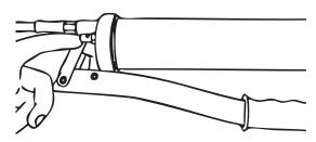
Remove air from the grease-containing section via the combined filling / air removal nipple on the grease gun head by loosening the gun head and cylinder (half a turn maximum) or by repeatedly actuating the hand lever.
